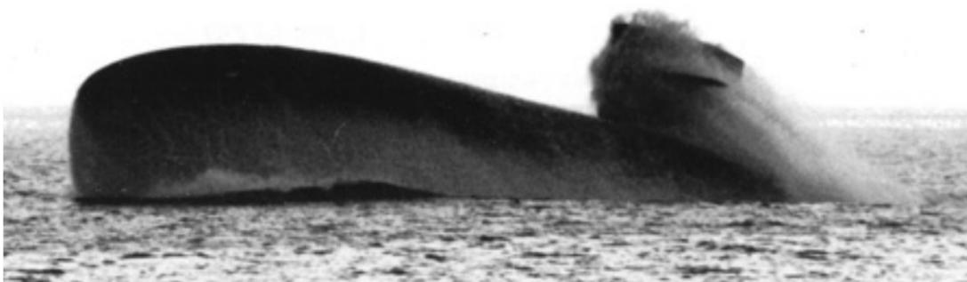
**The USS Philadelphia “breaching” after a test of its emergency blow system. The emergency blow system is designed to rapidly empty the sub’s ballast tanks and in doing so, force the sub to the surface.**
